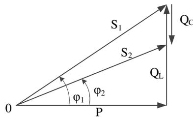
Fig. 1. **Opposite character reactive electrical power connection, vector diagram and PF change**
