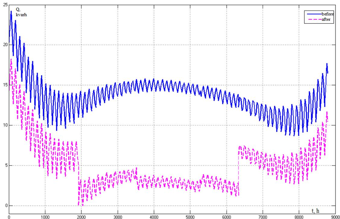
Fig. 7. Calculated reactive electrical energy in MatLab Simulink by ActC full method
